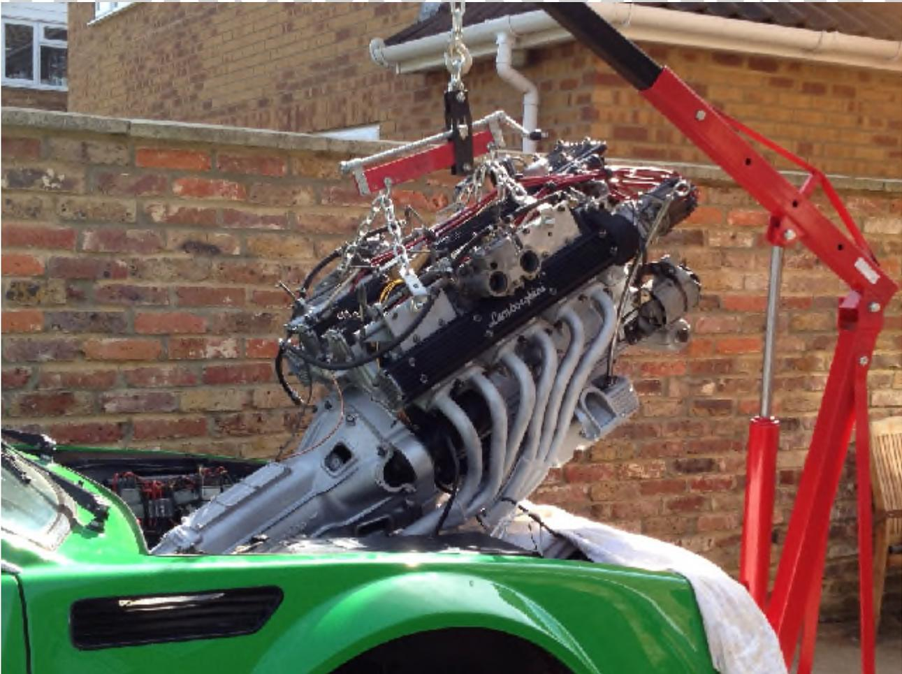
Look at the size of that thing! This was taken last year to replace the water pump and clutch. As one unit it is about 6 feet long.
